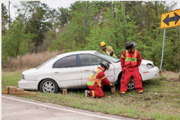
Stabilizing a car on its wheels with cribbing while patient contact is initiated.
