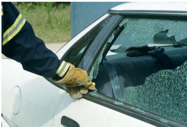
FIGURE 38-9 Using a spring-loaded center punch to break the window glass.
