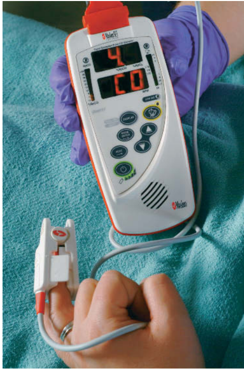
FIGURE 13-17 A CO-oximeter detects carbon monoxide as well as oxygen levels in the blood.
