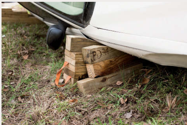
A vehicle on its side stabilized with cribbing.
