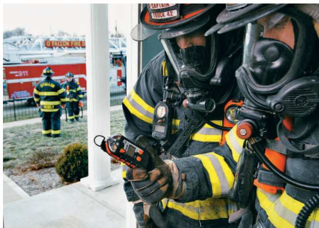
FIGURE 21-2 Special monitors are needed to detect the presence of carbon monoxide in the environment.
