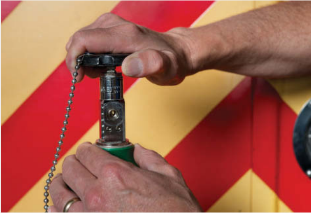
5. "Crack" the main valve for one second.
