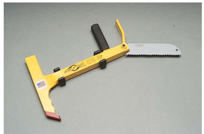
FIGURE 38-10 A Glas-Master saw can aid in windshield removal.
