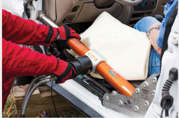
Use the spreader to roll back the dash.
