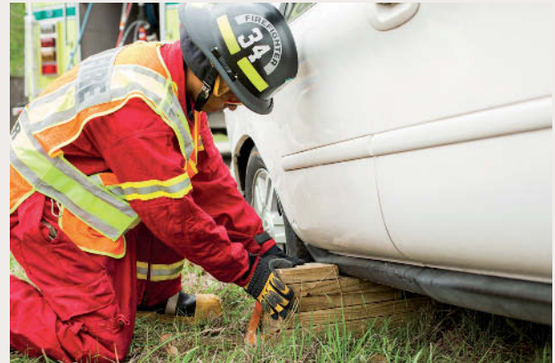
Placing a step chock. Keep hands clear of the vehicle while placing the chock.
