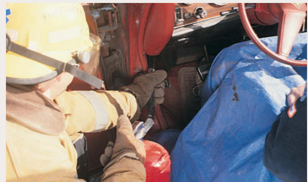
Extinguishing a fire under the dash. Care must be taken not to fill the vehicle's interior with a cloud of agent.
