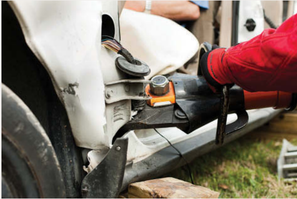
Make cuts for the spreader tool.
