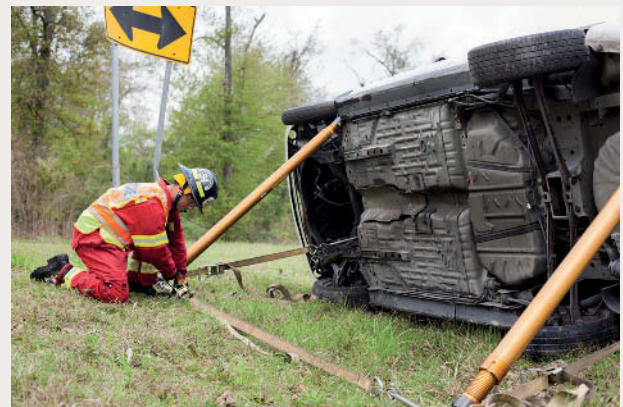
A vehicle on its side stabilized with struts. For maximum stability, it may be best to place cribbing on one side, struts on the other.
