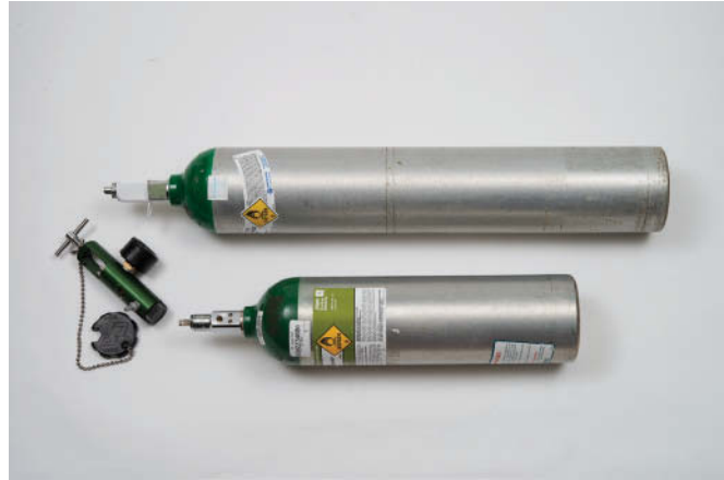
FIGURE 10-15 For safety, to prevent them from tipping over, oxygen cylinders must be placed in a horizontal position or, if upright, must be securely supported.
