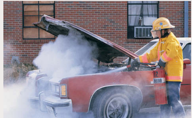
Extinguishing a fire in the engine compartment when the hood is fully open.
