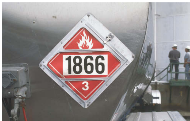
FIGURE 37-2 Vehicles carrying hazardous materials are required to display placards that communicate the nature of their cargo. Emergency Response Guides (ERGs) should be available to each emergency vehicle.
